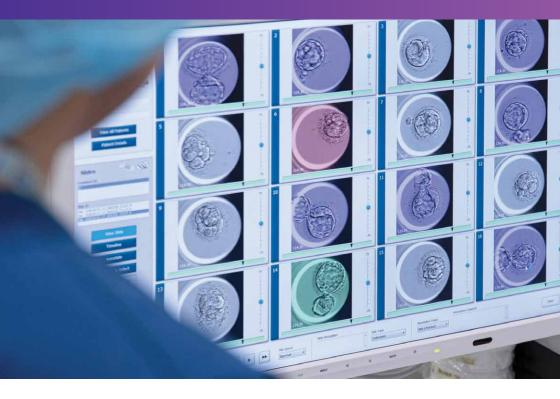
The EmbryoScope combines an incubator, high resolution camera and computer software to carefully monitor and analyse the development of embryos.
